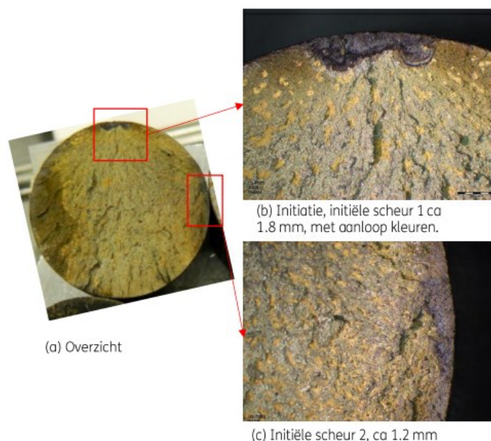
FIGURE 2: FRACTURE SURFACE OF STEEL REINFORCEMENT (BORSJE & SCHURING, 2023)
