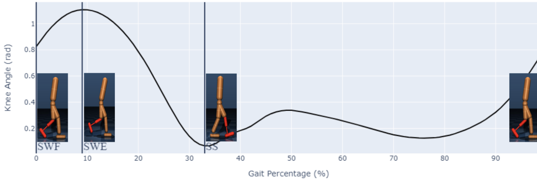
Figure 3.2.: Knee angle trajectory of a healthy human during level-ground walking. Divided into three phases, Swing Flexion (SWF) , Swing Extension (SWE) , and Stance (SS) .
