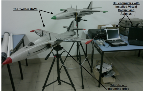
Fig. 1. Twister UAV (leader and follower) with HIL testbed setup.
