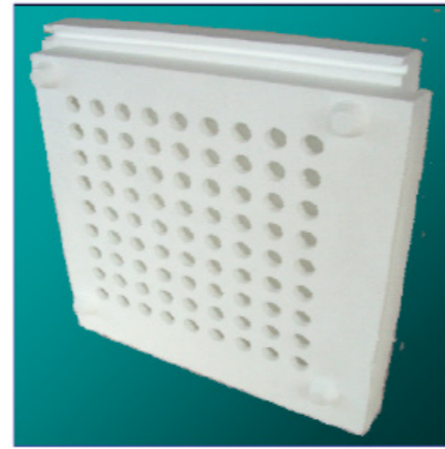
Figure 9: Parietodynamic wall construction. Source: A passive–active dynamic insulation system for all climates (p. 248).
