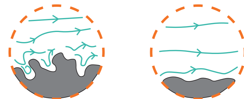
Figure 42: High surface roughness on the left creates eddies and possible backflows, while low surface roughness on the right does not induce a significant change to the flow. Source: Author.
