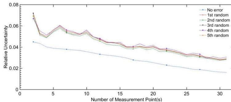
Fig.4. The relative uncertainty of the simulated irradiance measurement as a function of the number of measurement points for the Leipzig location. The lower curve is related to satellite-derived irradiance without adding error, the top curves are with an added simulated error.
