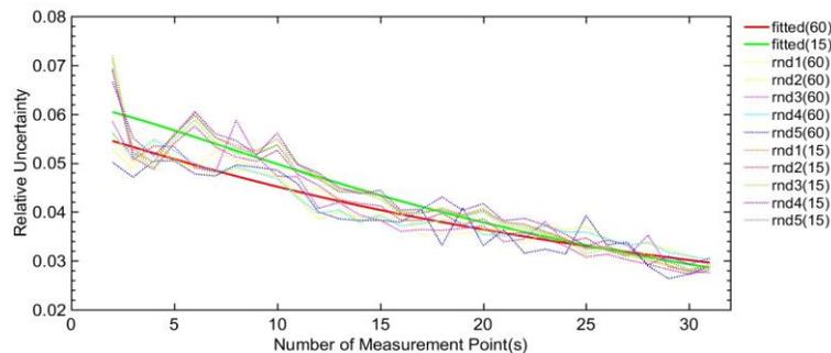
Fig. 6 Relative uncertainty in CSI as a function of the number of measurement points for two different temporal regimes. The green line is the fitted average of curves for 15-minute time-stamped data points, the red line is the fitted average of curves related to 60-minute time-stamped.
