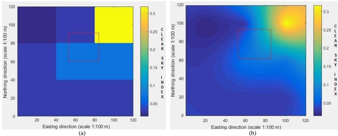
Fig. 2 (a) image of satellite derived clear sky index per pixel and (b) the interpolated clear sky index using the kriging method.
