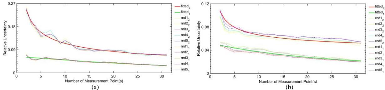
Fig. 5 Relative uncertainty in CSI as a function of the number of measurement points for the location in Leipzig (a) and Arizona (b). The bottom curves correspond to the small size measurement area, while the top curves correspond to the larger size measurement area.
