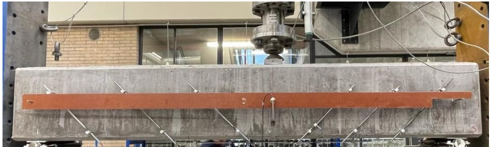
Figure 3.6: Picture after placing the LVDTs in one of the beams (front part)
