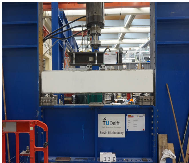
Figure 3.4: Actual test setup in the lab with a beam
