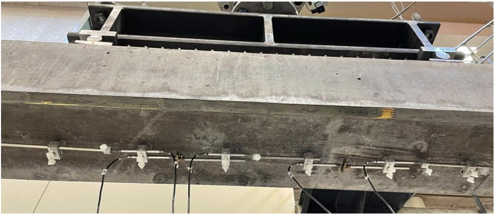
Figure 3.7: Picture after placing the LVDTs in one of the beams (bottom part)
