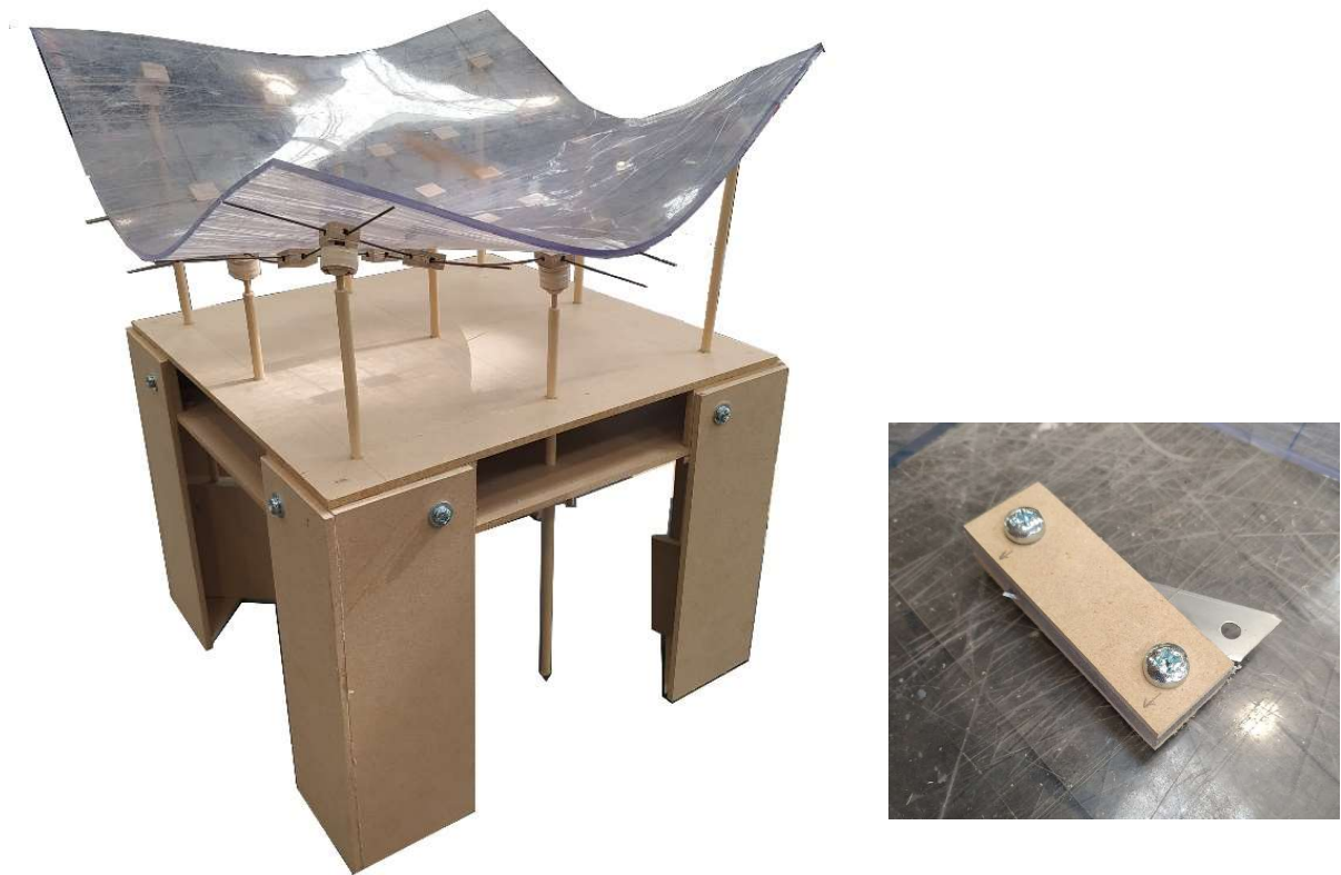
Figure 94 (a)The flexible surface on the grid, (b) The custom depth-cutting tool. Source: own illustration
