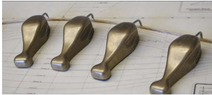
Figure 5 A thin birch strip (spline) fixed by hooked weights. Source: Edson International
