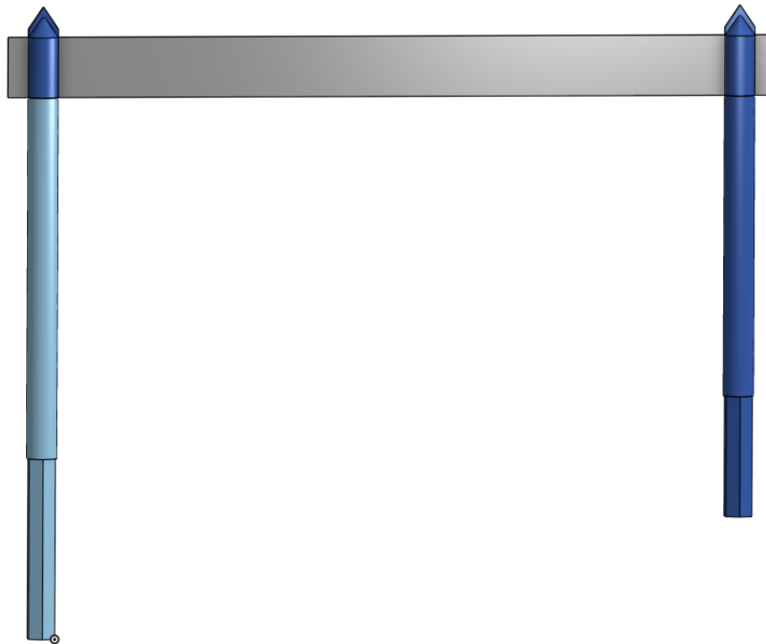
Figure 5.11: This figure shows the Preis-Device 2 with all the design iterations. It can be seen that the blade protrudes through both poles. The poles are changed as well, one is longer, and the other is shorter. This is to create space for the actuation mechanism being used manually and not hinder the movement of the other pole. Another iteration concerning the poles is the hexagonal shape towards the end of the poles. This is done in order to fasten the actuation mechanism to the poles in an easy manner. The last iteration that can be seen is the tip of the caps. Instead of the caps being tapered, a blade-like ridge has been incorporated in order to facilitate cutting and insertion of the device. This figure was created using Onshape (Onshape Inc., Massachusetts, USA)
