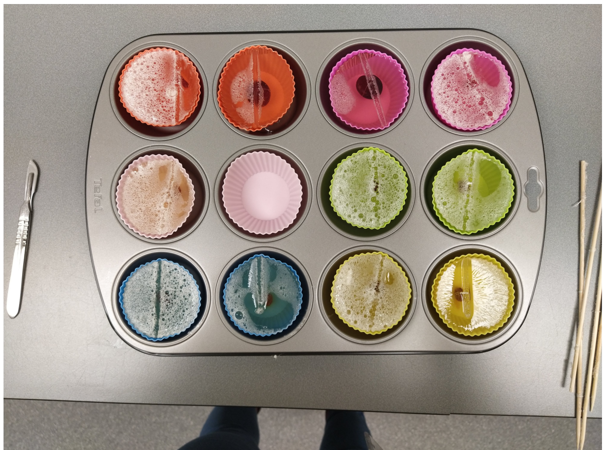
Figure F.1: This figure shows the phantoms made in the cupcake forms. These phantoms have already cooled for 24h in the fridge at 6°C. After warming up to room temperature, they are ready to be used
