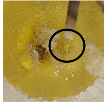
Figure 4.7: This figure shows the insertion cannal (inside the black circle). The blade is held for reference, showing that the insertion cannal is less than 5\text{mm} in diameter. This cannal was made with a 0.04\text{mm} blade. The picture was taken by the author
