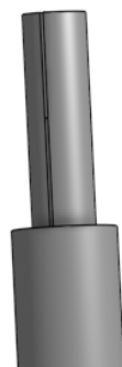
Figure 3.2: This figure depicts the distal end of the pole. It shows the 0.1\text{mm} slit the blade cut out fits into. It can also be seen that the milled down end of the pole, 1\text{mm} in diameter, which accommodates the cap. Both poles are fabricated the same. This figure was created using Onshape (Onshape Inc., Massachusetts, USA)
