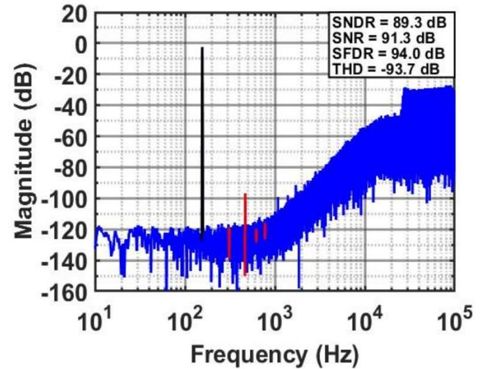
Fig. 4. Measured output spectrum at 200 kHz  $f_s$ .
