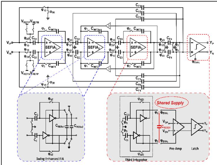
Fig. 1. Circuit schematic of  $\Delta\Sigma$  Modulator
