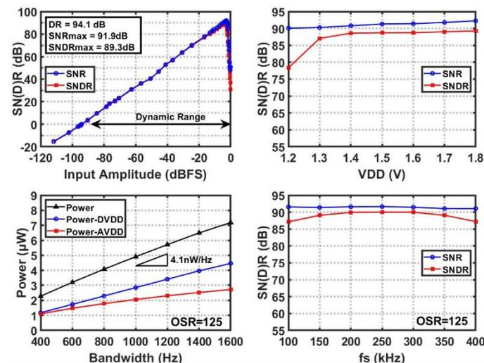
Fig. 5. (Top left) SNDR/SNR vs. input amplitude, (top right) SNDR/SNR vs. VDD, (bottom left) power consumption vs. Bandwidth, and (bottom right) SNDR/SNR vs.  $f_s$  when OSR=125.
