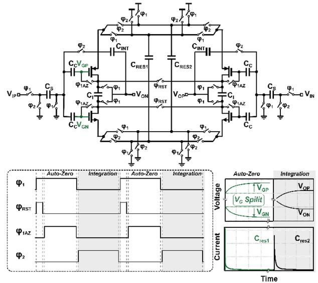
Fig. 2. Simplified circuit diagram of the proposed SEFIA and the corresponding timing diagram.
