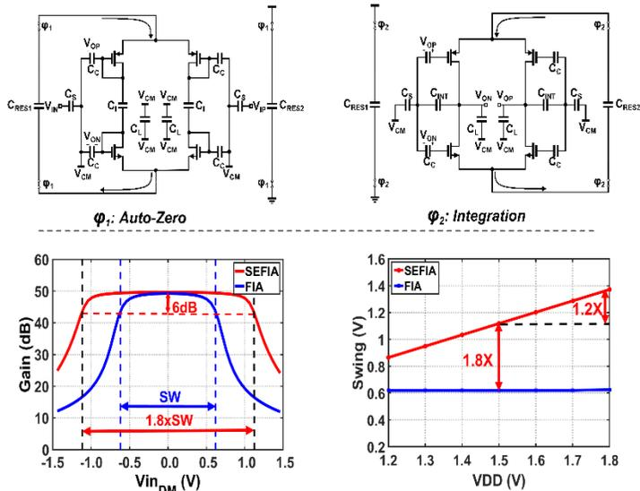
Fig. 3. Operation and output swing comparison of the proposed SEFIA and conventional FIA.
