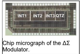
Chip micrograph of the  $\Delta\Sigma$  Modulator.
