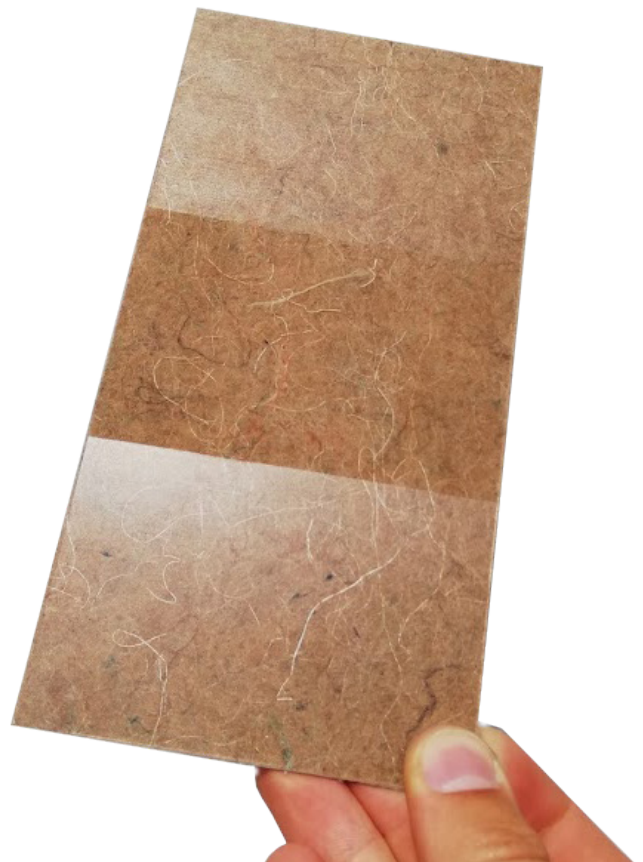
Figure 41: N9010 jute sample pressed with aluminum plate
