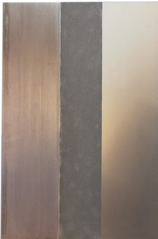
Figure 40: Aluminum plate with, from left to right, a textured, mate and satin finish
