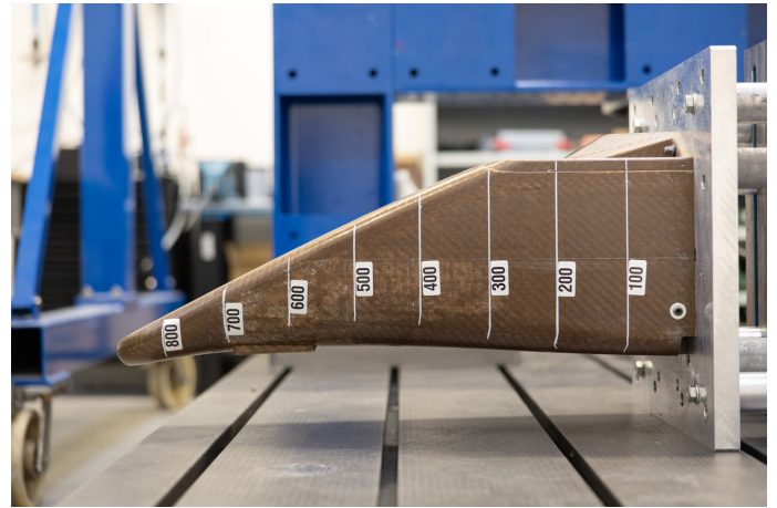
Figure 8: Flax composite formula crashbox, Source: Maher, 2020
