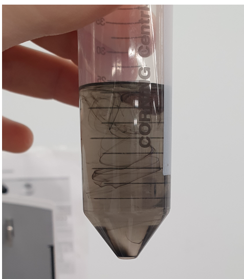
Figure 21: Redispersion of graphene into supernatant.
