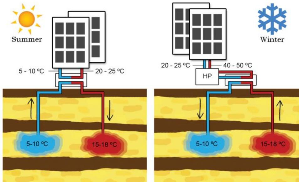
Figure 2. ATEs-doublet working principle
