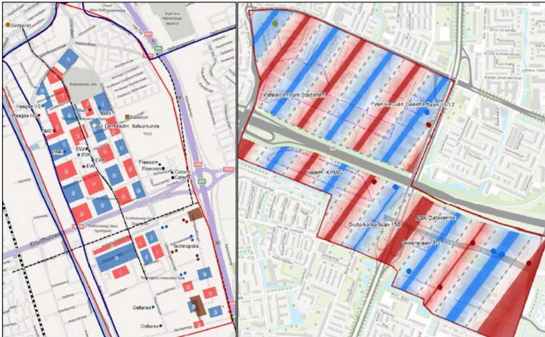
Figure 1A cut out of the ATES plan maps in Delft (left) and Amstelveen (right), indicating search areas for warm and cold well (the red and blue areas) and existing well locations (green, red and blue markers).
