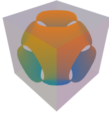
(b) Fermi surface after adaptive sampling. The isosurface consists of 11640 triangles.
