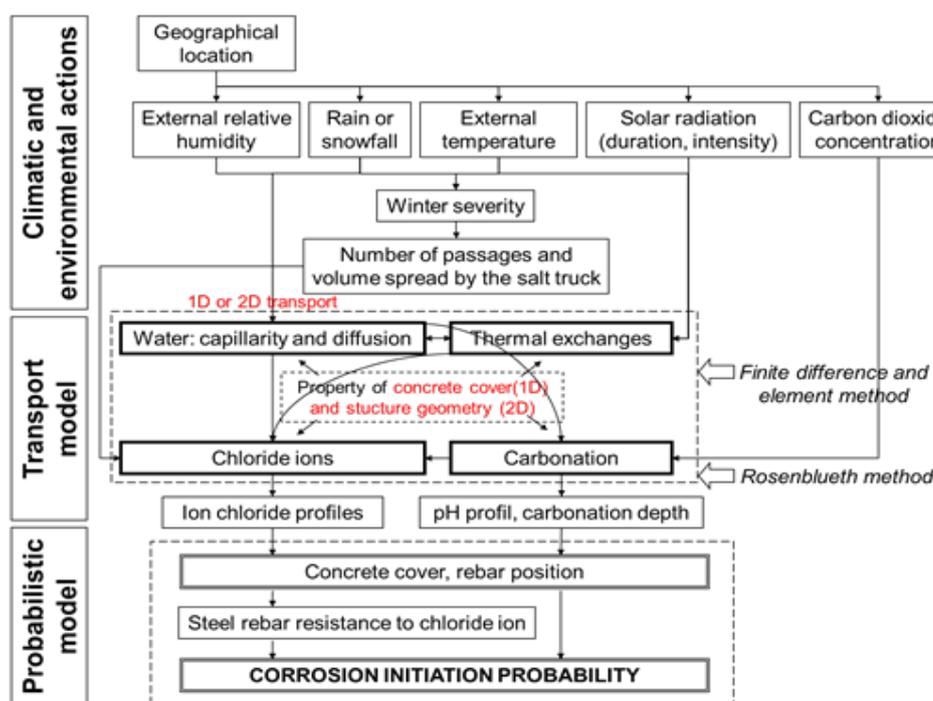
**Figure 1: Implementation of a new 2D water transport module in the TransChlor<sup>®</sup> software architecture**
