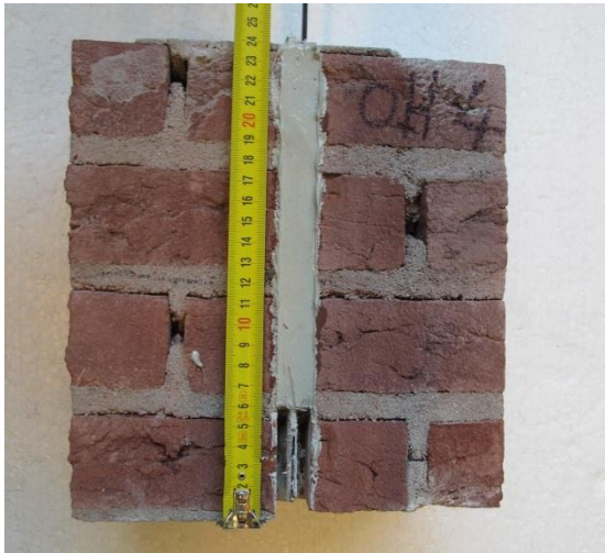
Figure 59: A sample form the pull-out tests performed by the TU/e [46]
