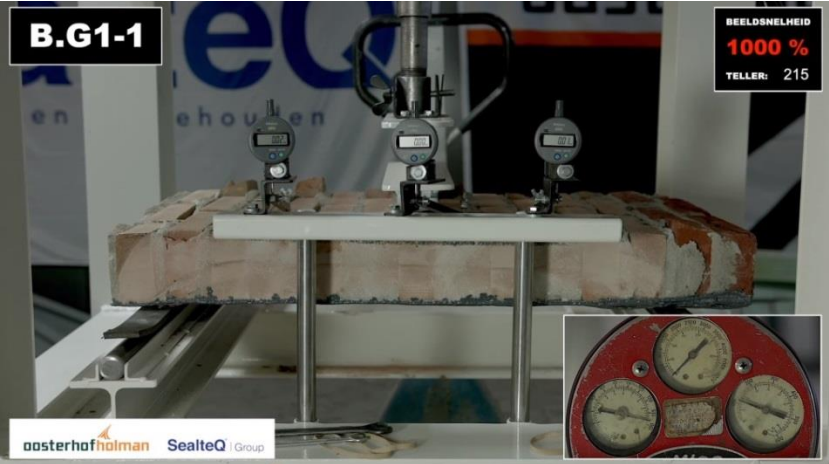
Figure 45: Test setup used for the OP bending test (screenshot taken from a Youtube movie of the Quake-Shield Youtube channel [43])
