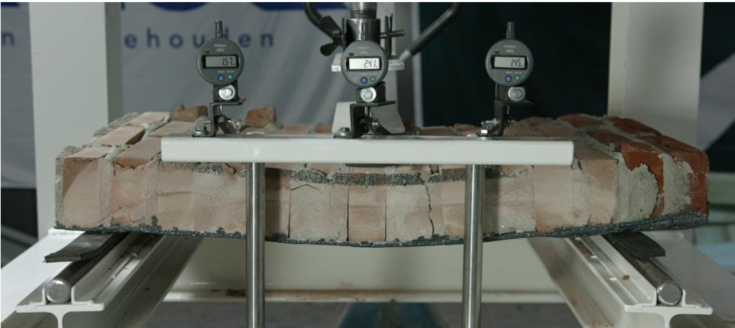
Figure 76: Test sample (BG1-1) at 24,1 mm displacement [43]
