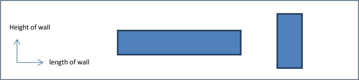
Figure 9: Examples of aspect ratio. Left: low aspect ratio (<1), Right: high aspect ratio (>1)
