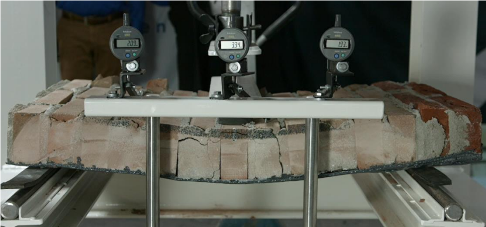
Figure 80: Test sample (BG1-1) at 33,4 mm displacement [43]
