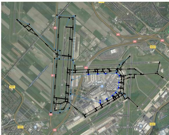
Figure 6: Overlay of the nodal network on a satellite image of Amsterdam Airport Schiphol.
