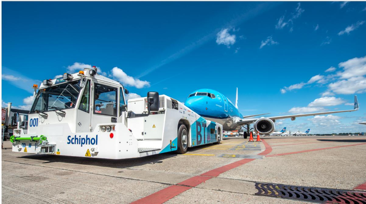
Figure 4.8: TaxiBot taxiing an aircraft at Schiphol during the Proof-of-Concept test in 2020 [5].
