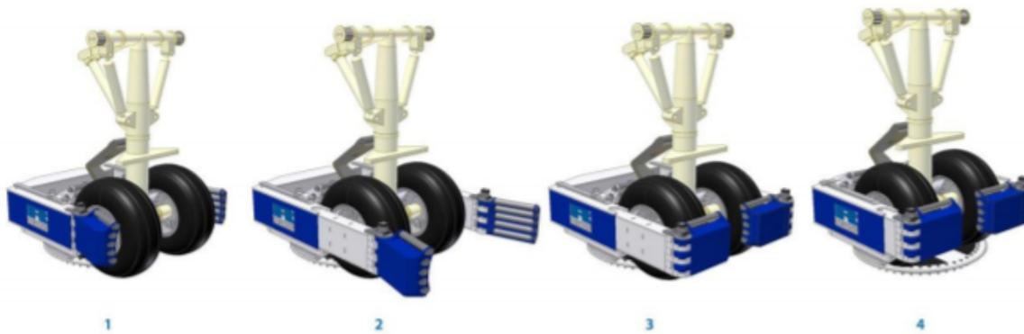
Figure 4.9: The four steps in which the NLG enters the vehicle turret and gets clamped securely in position [26].
