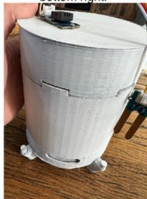
Disconnect cable and put top on the housing.
