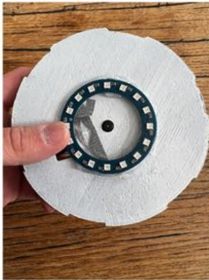
Hot glue LED ring to bottom of the housing plate.
