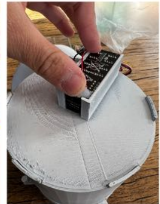
Secure Grove shield to housing, make sure the camera fits in the middle hole.
