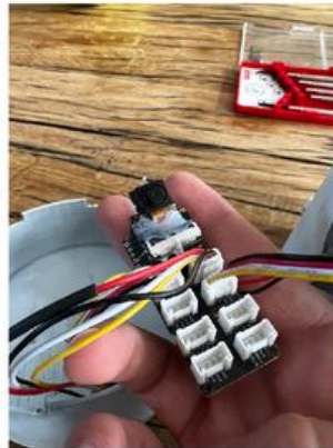
Connect electronics, top left DHT20, top right moisture meter and LED bottom right.
