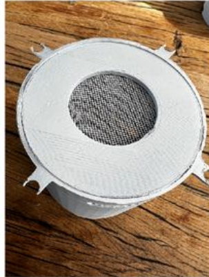
Secure mesh in middle part of Cephal.
