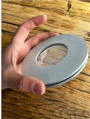
Secure mesh between holders, use hotglue if needed.
