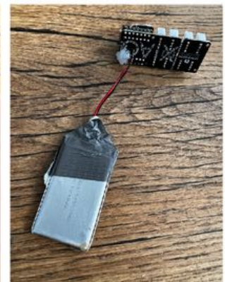
Solder battery to grove shield.
