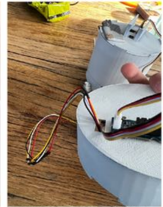
Put cables of both the DHT20 and moisture meter through hole.
