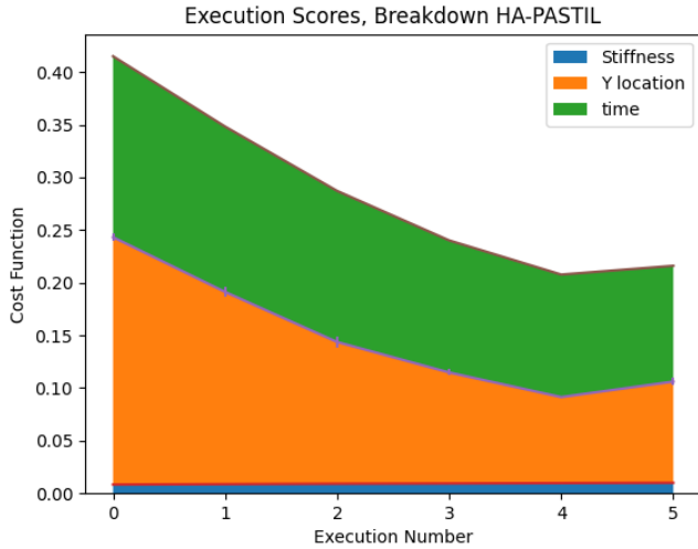
Figure 5.3: Breakdown of the cost for HA-PASTIL on the Push task. The green part represents the time it takes for the box to be pushed off the table, while the yellow part represents the distance of the final position of the box to the table. The blue part represents the cost for the stiffness.
