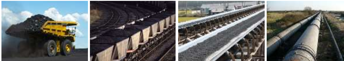
Figure 4-4: Options for transport, A. Truck, B. Train, C. Conveyor belt and D. Slurry pipeline
