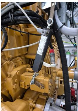
(a) The installed throttle position sensor (TPS). Connected to the shaft of the throttle actuator that also actuates the throttle linkage
