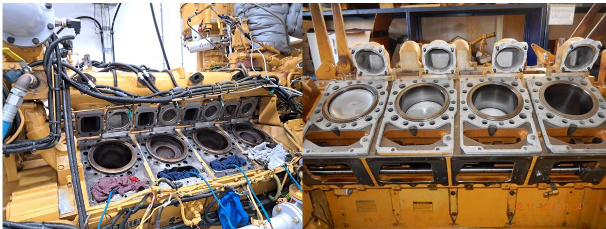
(a) The CAT G3508a engine at the NLDA in Den Helder with the individual cylinder heads removed of bank 2, notice the bowl shaped pistons.
