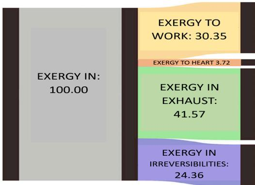
(a) Sankey diagram illustrating how the ingoing exergy is transferred due to work, via heat transfer, via the exhaust gases, and destroyed due to irreversibilities in the high-pressure phase of the engine operating cycle[22]
