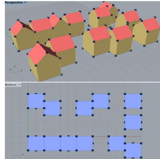
Check if Input Lists of Attributes are successfully assigned to corresponding HBSurface and HBZone.
