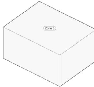
0.06 Each surface of the zone is modeled as a flat plane, which will later be labeled with names and assigned properties.
