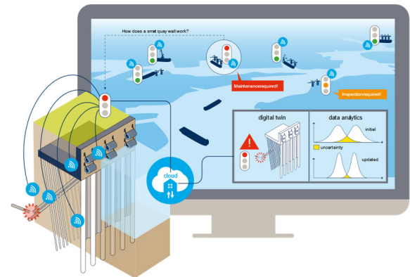
Figure 2. Concept of a smart quay wall (Roubos, 2019).
