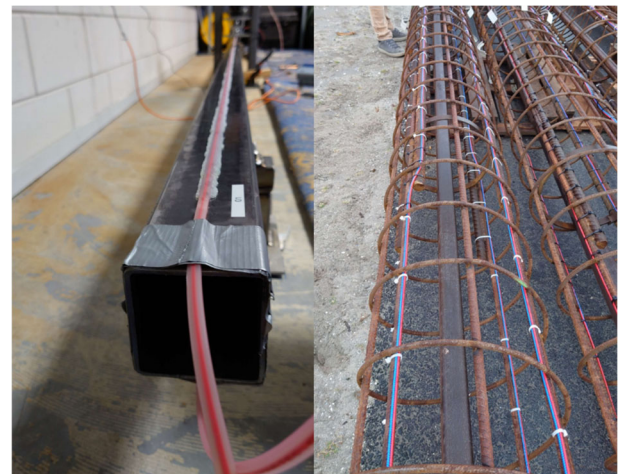
Figure 4. Impression fibre optic strain sensors.
