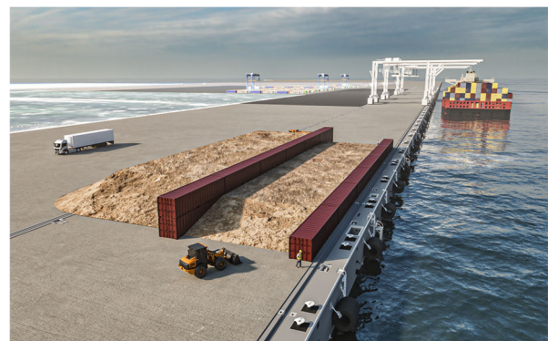
Figure 7. Preparation for the full-scale field test of the quay wall at Maasvlakte 2, scheduled to begin in Q3 2025.
