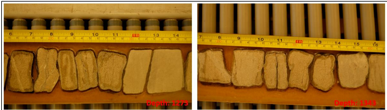
Figure 30 Cores of Alblasserdam Member at Well Bleskensgraaf-2 (BLG-02) at depth -1273 m and -1343 m
