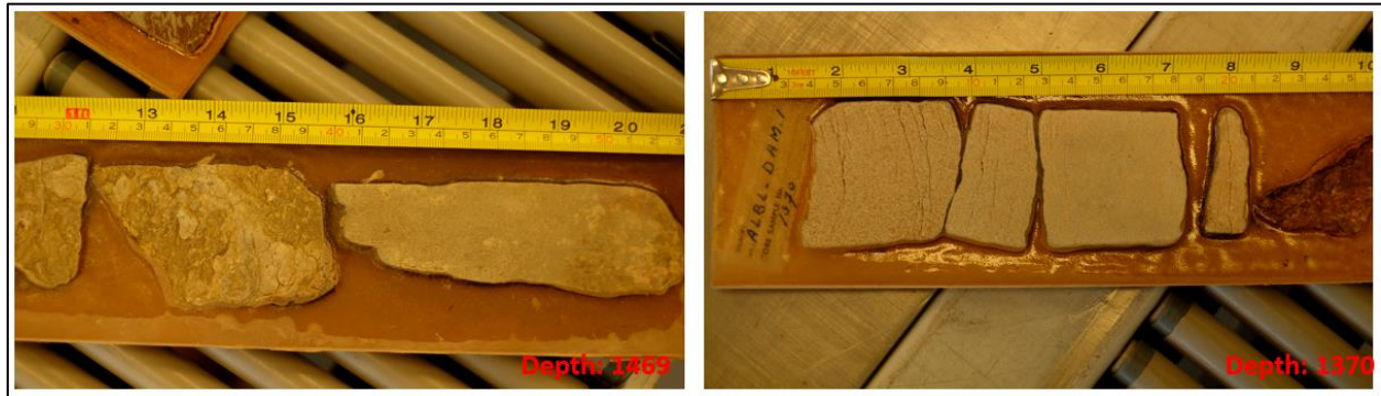
Figure 32 Cores of Alblasserdam Member at Well Alblasserdam-1 (ALD-01) at depth -1469 m and -1370 m
