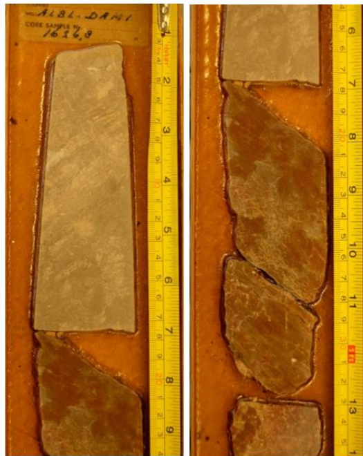
Figure 56 Oxidized siltstone core of SDLNA in well ALD-01
