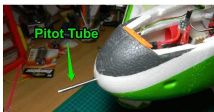
Figure 3.2: Fixed wing aircraft have the advantage of placing pitot tubes in free-stream velocity air.
