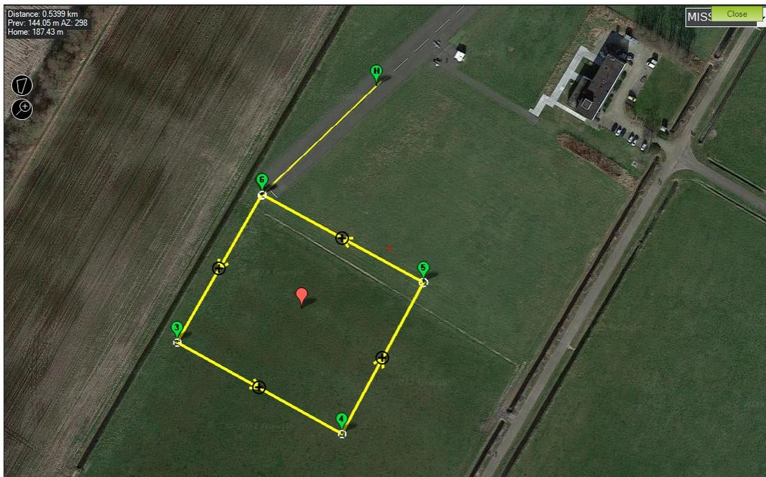
Figure 5.1: Exemplary flight plan at Marknesse location. Subject to change as the square is supposed to be exactly perpendicular to the wind direction.
