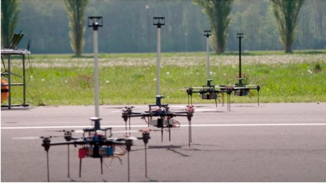
Fig. 1. Foxtech Hover 1 drones used in this research, with wind sensor mounted on top at a distance from rotor air flows. The proposed methods in this paper estimate wind without the use of the shown sensors.
