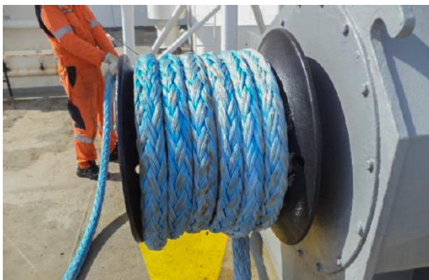
Image 2.14: A Dyneema® rope in use, the grey color on the ropes indicate contaminations on the rope. Source: (Dynamica-ropes.com, 2019).
