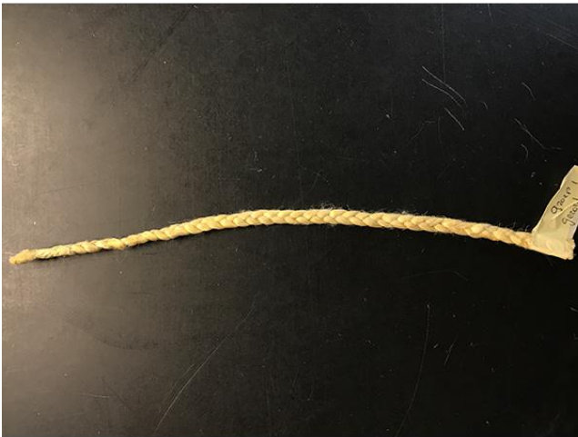
The softened rope from the uncovered rope was easy to braid and is of similar quality compared to the new rope.
