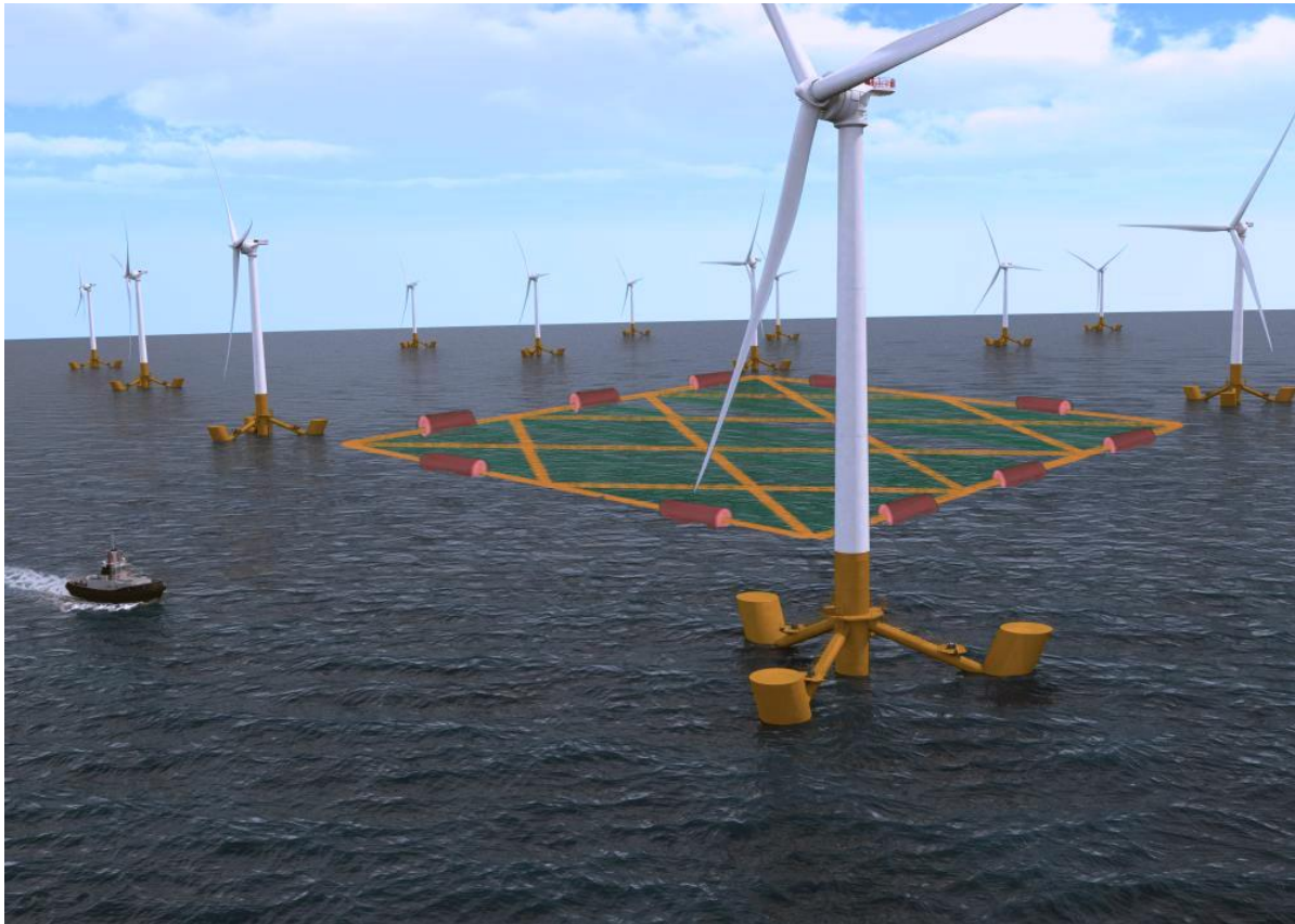
Graphic 6.6: The final re-design, the seaweed farm is positioned between windmills that double as anchor points. The buoys, in red, are for the needed buoyancy. Source: self-made graphic.
