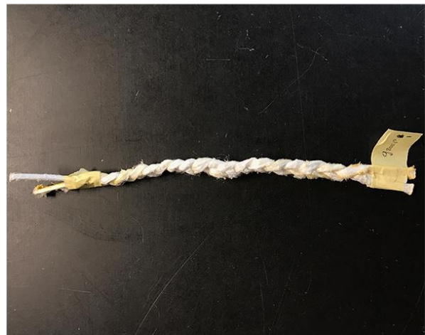
Graphic 3.6: The yarns were braided into ropes to test get an idea of how the yarns could be used, the rope was very poor quality due to the stiffness of the yarn. Source: self-made image.
