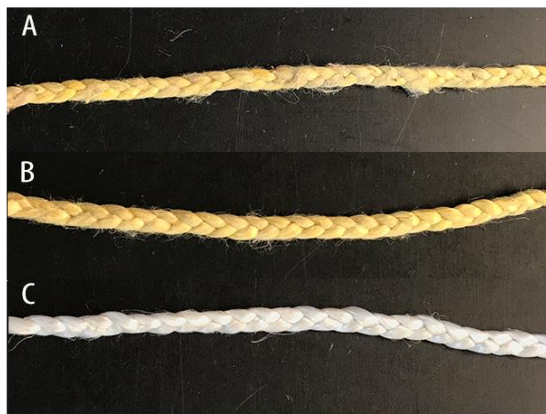
Three ropes of different quality. A is a rope made from poor condition EoU yarns. B is made from good condition EoU yarns. C is made from new yarns.
