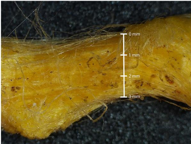
Yarn of the unshielded rope, the dark yellow indicates the presence of a coating. Also note the contaminations that are present, see the black spots.
