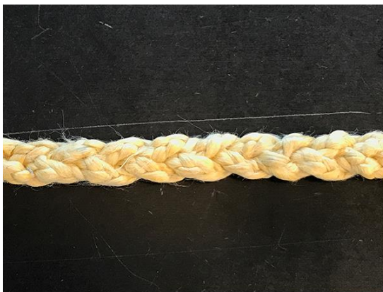
A rope braided from other ropes as a way to possibly reduce the time needed to take the ropes apart..
