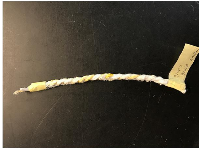
The yarn from the covered rope was still hard to braid and it resulted into a poor quality rope compared to the new rope.
