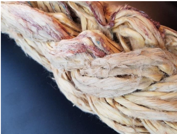
Image 3.1: An uncovered Dyneema® rope, fluffy fibers from abrasion damage and contamination from paint and oil can be seen here. Source: self-made picture.
