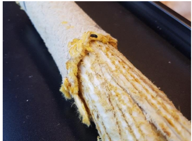
Image 3.2: A covered Dyneema® rope, at first sight this rope looks less damaged and contaminated. Source: self-made picture.
