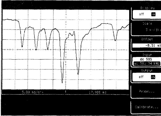
Figure 3.9 Superposition of consecutive discharges for voids with a large D/h ratio, D=20 mm, h=1 mm.
