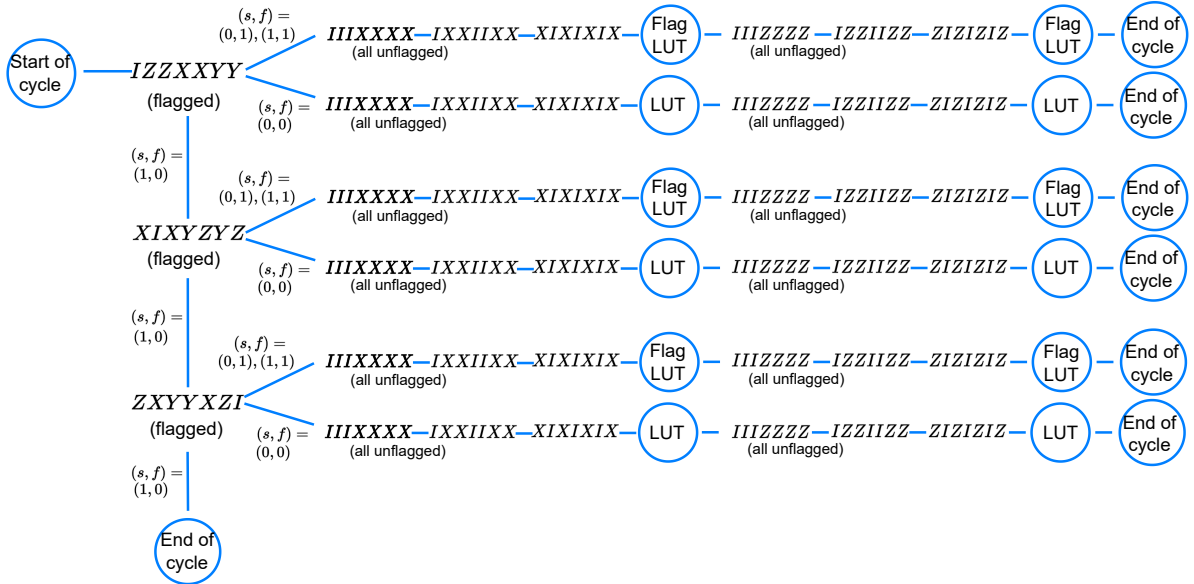
Figure 5.7: The detect-and-diagnose flag protocol for the Steane code. This protocol requires 3 weight-6 flagged stabilizer measurements, instead of the 6 weight-4 generators required by the original protocol in Fig. 4.6.
