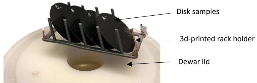
Figure 2. The setup for the cryogenic thermal cycling of the samples.
