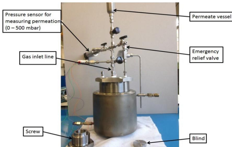
Figure 3. A view of the permeation setup.
