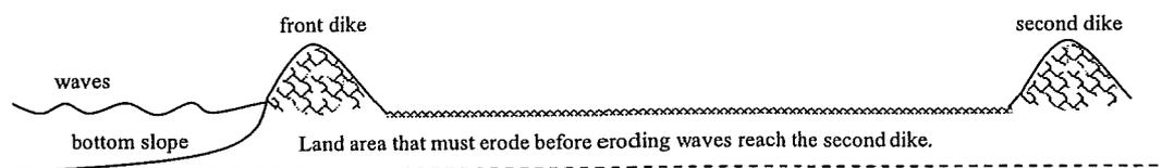
**Figure 4.4** Simple sketch of Van Ly dike situation.
