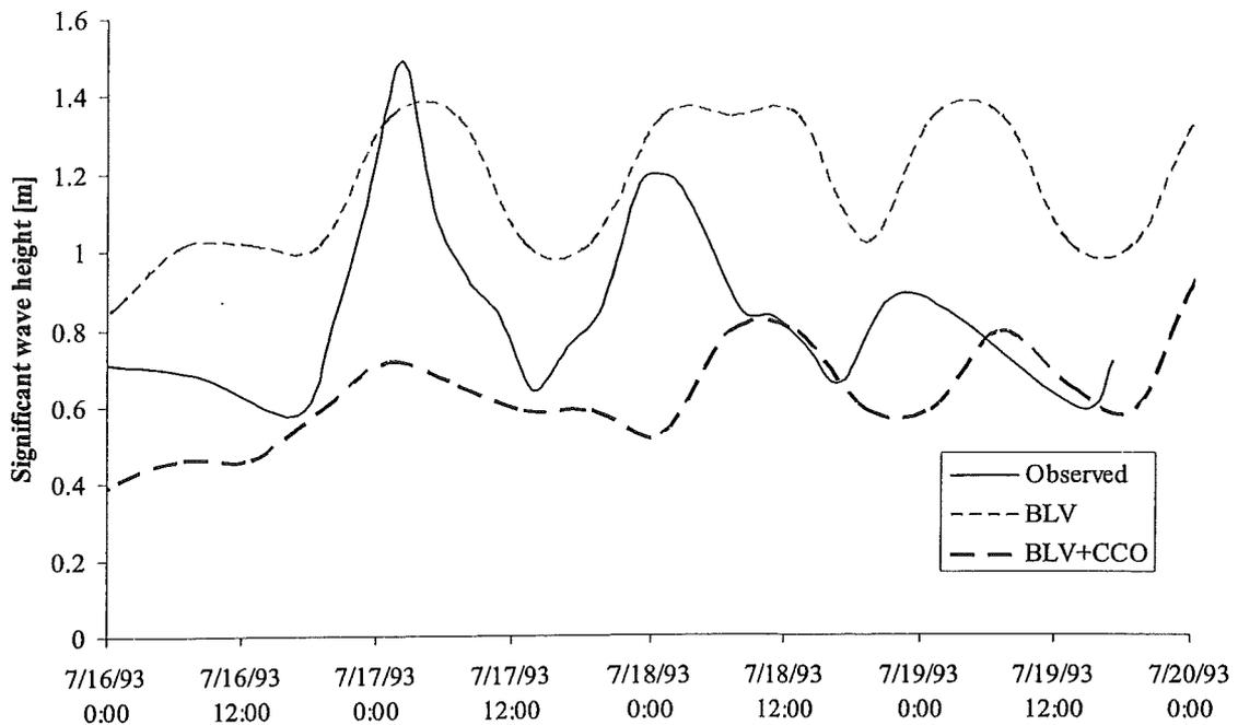
Figure 4.15 Observed and calculated waves outside Van Ly in July 1993 (waves from the south).
