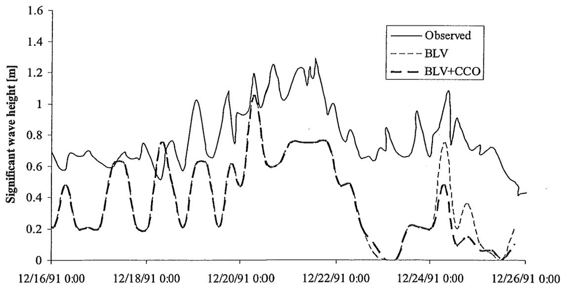
**Figure 4.14** Observed and calculated waves outside Van Ly in December 1991 (wave from the north).
