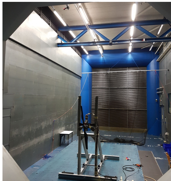
Figure 1: The new DelftaCopter Propulsion System is mounted on a static test rig in the TUDelft Open Jet windtunnel. The test setup includes force measurements, moment measurements, voltage, current, airspeed, rotor pitch, throttle and rotor rpm measurements.
