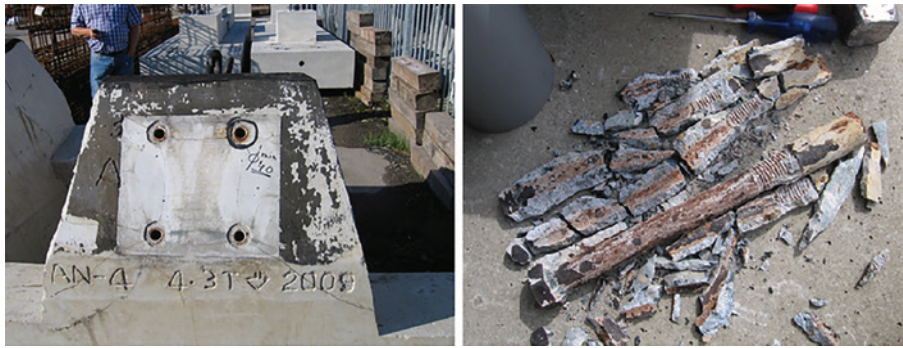
Figure 9: Damaged block due to the corrosion of anchor induced by stray current.
