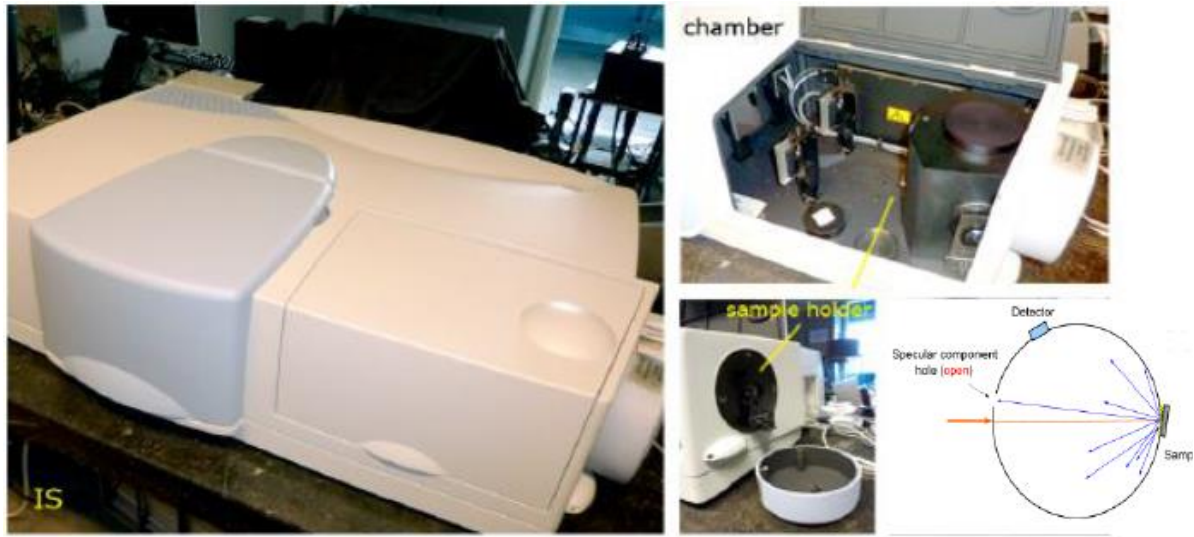
Figure 23: The Integrating Sphere setup [48]
