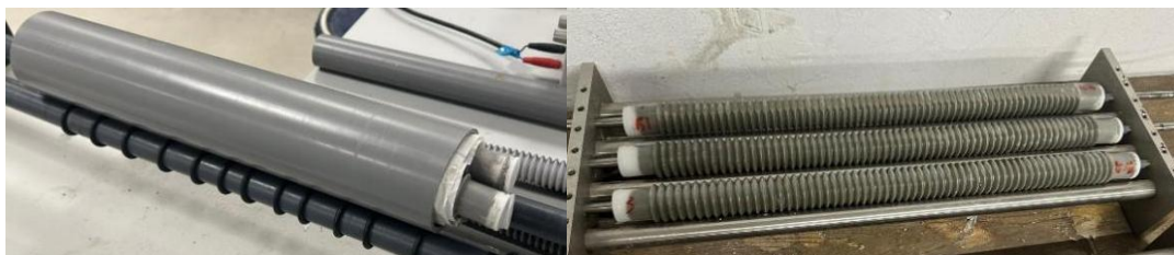
Figure 3.5. Rotation machine (left) and autogenous shrinkage test device (right).
