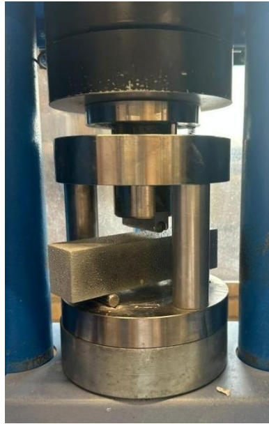
Figure 3.4. Setup for flexural strength test (three-point bending test).
