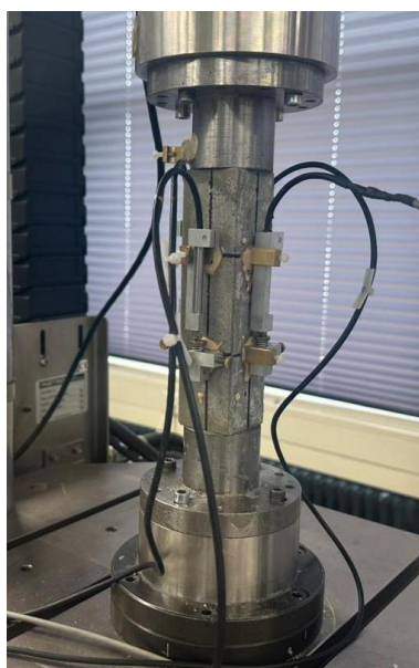
Figure 3.3. Setup for E-modulus test.
