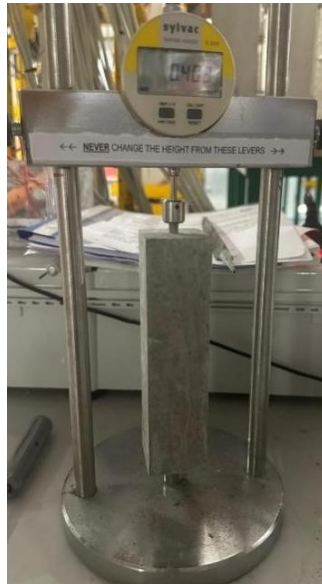
Figure 3.6. Setup for drying shrinkage measurement
