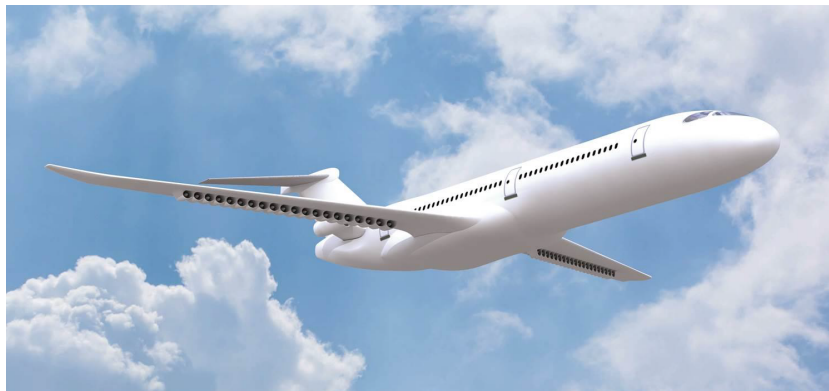
Figure 1.5: ONERA's hybrid-electric DRAGON concept [5].
