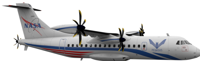
Figure 1.4: NASA's PEGASUS concept: a retrofitted ATR 42-500 using wingtip propulsors and BLI [4].
