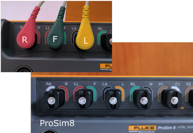
Figure 5.5: Connection of 6 different patient monitors to Frankie and one example of connection to ProSim 8.
