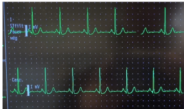
Figure I.3: Lead I, II and III detected by GE Healthcare patient monitor when the Prototype's outputs are connected to electrode cables as: GND to F; V- to R and V+ to L.
