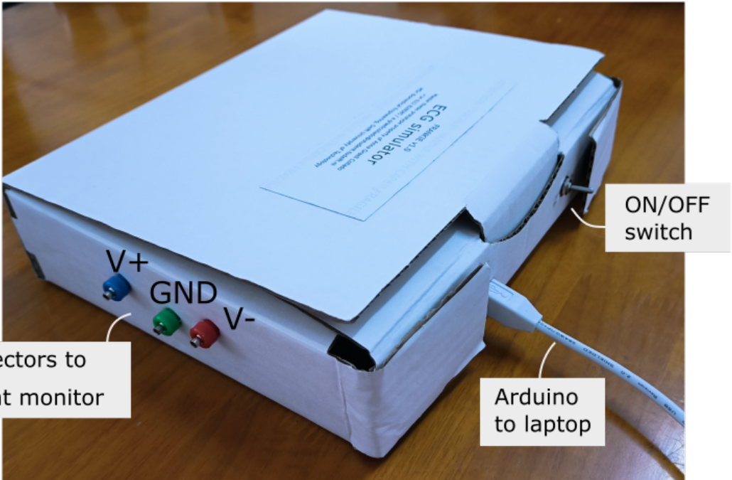
Figure 5.4: Images of Frankie's outer casing and inside electronics. The white cable is used to connect the Arduino to a laptop when the user wants to modify the simulated waveform.
