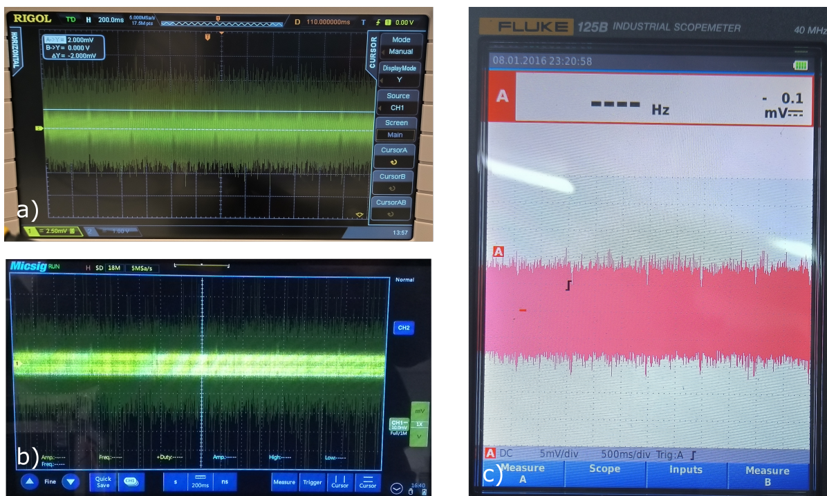
Figure L.1: ECG-like waveforms in the millivolt range detected by three common oscilloscopes. a) 2 mVpp ECG waveform generated by 214A commercial simulator as detected by Rigol DS2072A Oscilloscope (2.5 mV/div). b) 1 mVpp ECG waveform generated by the Prototype (PWM + LPF + voltage divider) as detected by Tablet Oscilloscope tBook mini TO1000 (10 mV/div). c) 5 mVpp ECG waveform generated by ProSim 8 as detected by Fluke 125B Industrial Scopemeter (5 mV/div).
