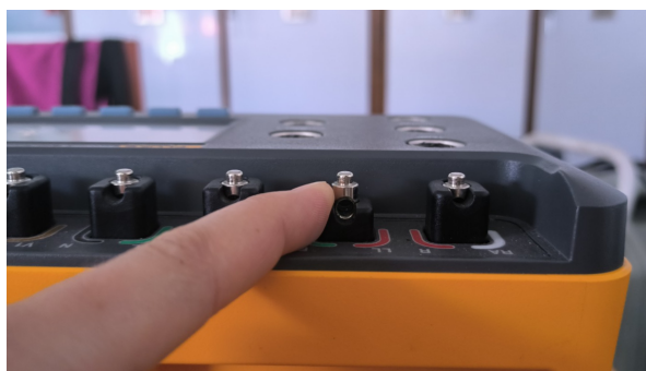
Figure 6.4: ProSim 8 features specialized connectors the tip of which resembles ECG electrodes.
