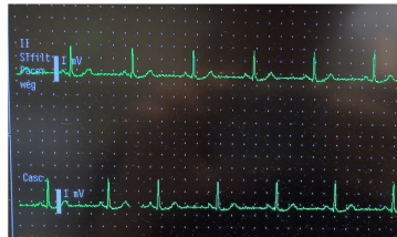
Figure I.3: Lead I, II and III detected by GE Healthcare patient monitor when the Prototype's outputs are connected to electrode cables as: GND to F; V- to R and V+ to L.
