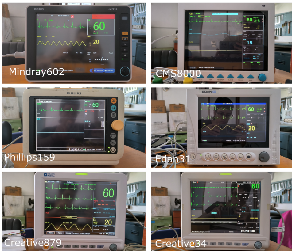
Figure 6.5: Connection tests: Prototype and ProSim 8 connected to 6 different patient monitors at Green Pastures Hospital (Pokhara, Nepal). Simulators were set to generate a 60 bpm, 2 mV ECG-like waveform in all cases except for Creative879 (60 bpm, 3 mV).
