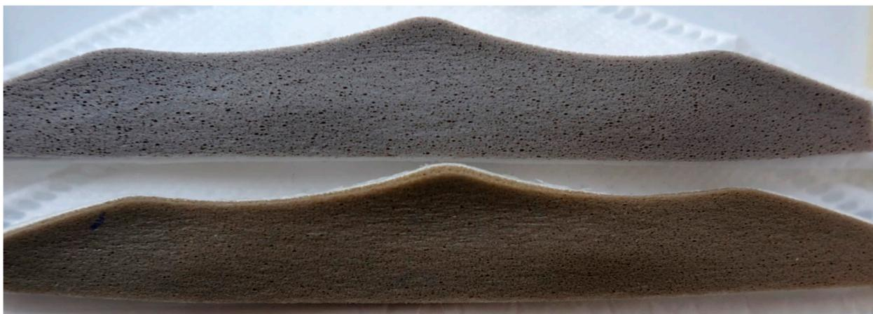
**Figure 8.** Nose comfort cushion after different ClO<sub>2</sub> sterilisation cycles (Top: 0 cycles, bottom: 6 cycles).
