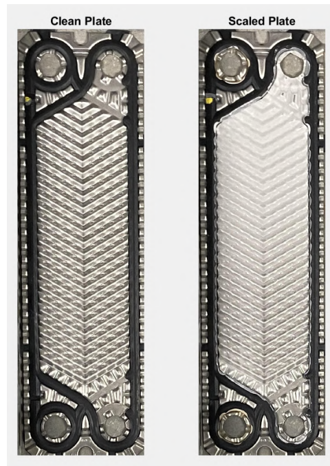
Figure 33: Comparison of the first scaled plate vs clean plate for the base case
