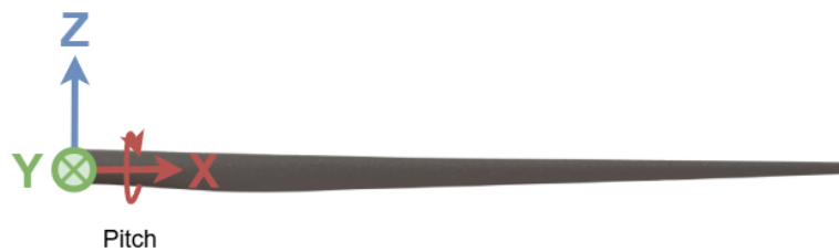
Figure 3.9: Schematisation of the offshore wind turbine blade with indicated local coordinate axes.
