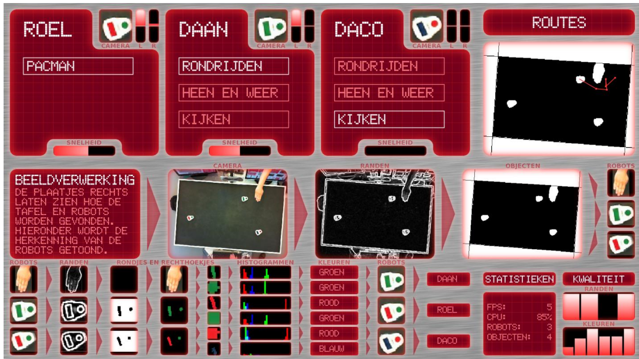
Figure 9-2: The right screen of the GUI showing the AI states, image processing, path finding and the quality of service
