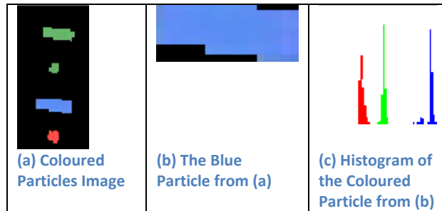
Figure 6-3: Image Processing: extracting colours
