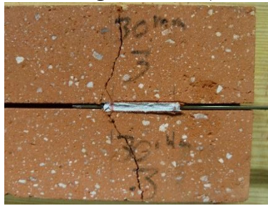
B (Full debonding with diagonal cracks)
