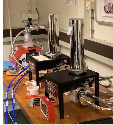
Figure 3.5: The outside of a cryostat.
