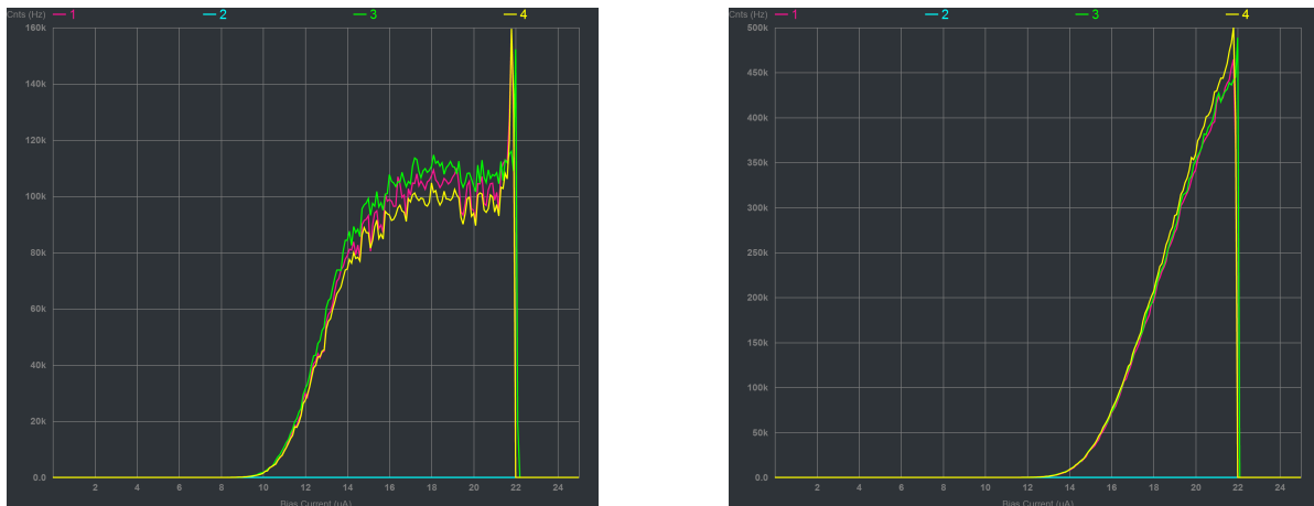
Figure 4.3: The IC-curves of a 4-pixel SNSPD in a cryostat under flood illumination by laser light with a wavelength of 780 \text{ nm} (left) and 1300 \text{ nm} (right). The different colours correspond to the different pixels. Three out of four pixels work. The vertical axis represents the number of counts. The horizontal axis represents the bias current.
