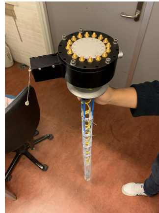
Figure 3.7: A dipstick after measurement. The dipstick has just been removed from a container of liquid helium and at the bottom the PCB is still attached.
