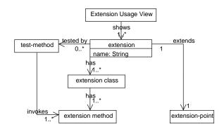
Figure 5. Meta Model: Extension Usage View
