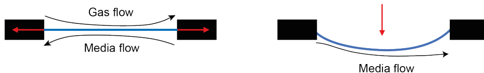
Figure 2.9: Schematic illustration of media and gas flow alongside an in-plane stretched membrane and an out-of-plane stretched membrane. Red arrows indicate the stretching direction.
