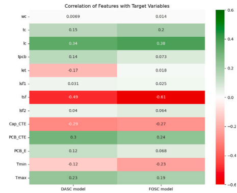
Fig. 5. Correlation matrix of input features to outputs of DASC model and FOSC model.
