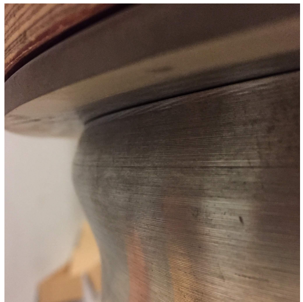
FIGURE 11: PLASTIC DEFORMATION AT THE EDGE OF THE CYLINDER.
