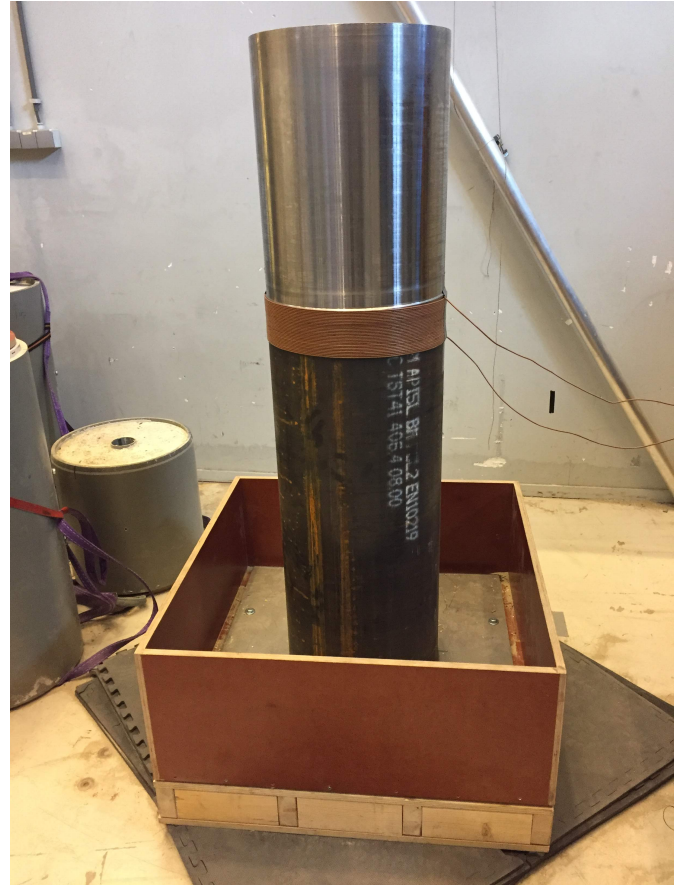
FIGURE 2: THE CYLINDER WITH INSTALLED COIL.
