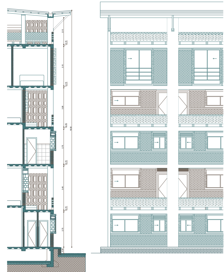
Figure 99 Detail section facade.
