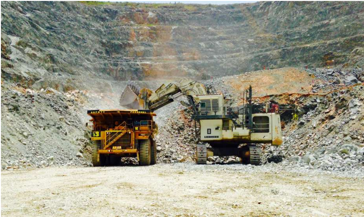
Figure 2.13: A Liebherr 9400 Face Shovel loading a Caterpillar 785C Truck in the Subika pit
