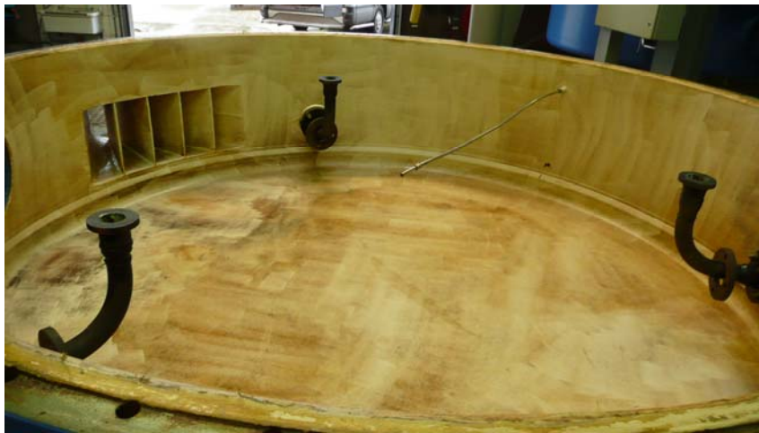
Figure 8: Three pellet discharge points at the bottom of reactor
