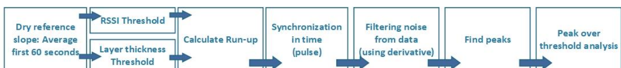
Figure 20 Overview of the steps taken to obtain the wave run-up height distribution
