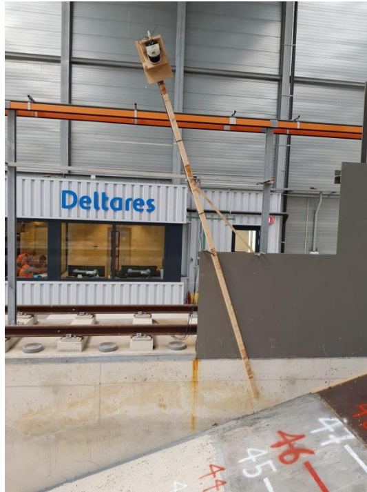
Figure 12 Positioning of the laser scanner on the wall of the flume (Çete, 2018).
