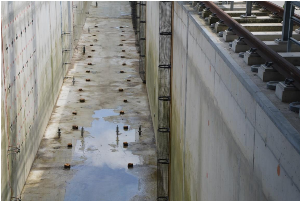
Figure B.4 The configuration in the flume during the reference tests, only a small part of the stem of the willows is left
