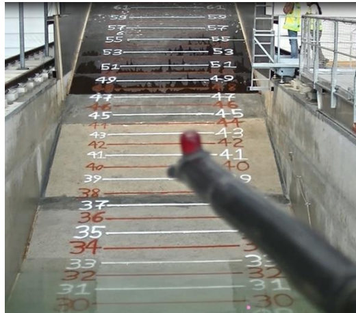
Figure 30 Synchronization LED light (Çete, 2018)
