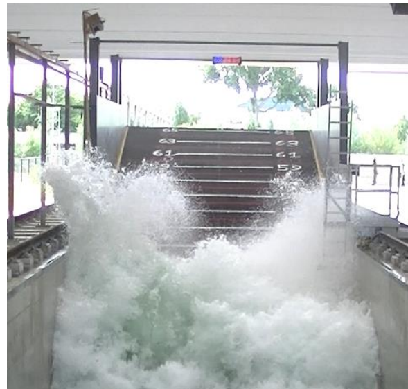
Figure 61 Wave breaking on the dike measured by laser and by camera, for test T041
