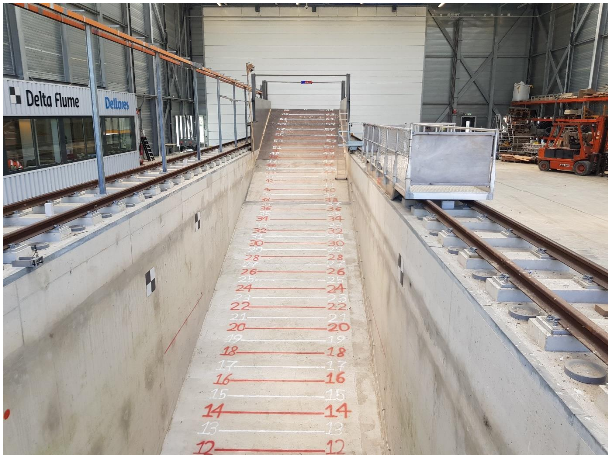
Figure H.1 Slope of the dike in the delta flume with the painted lines (Source: Deltares, 2018).
