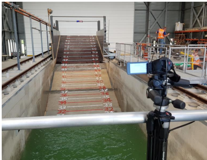
Figure 13 The video camera positioned on the walking bridge pointing to the slope of the dike (Çete, 2018)
