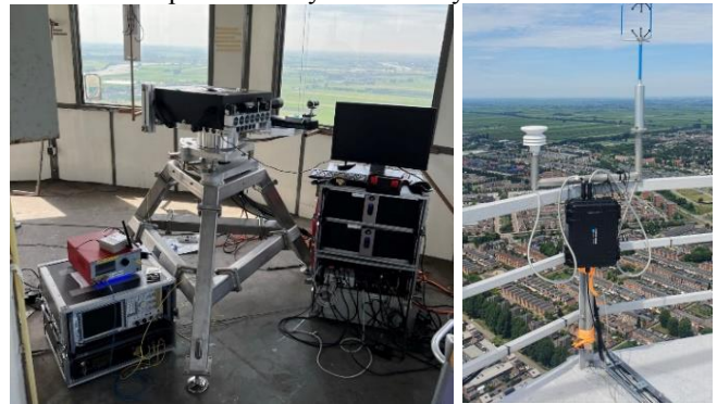
Figure II-2: STB located in the crow's nest (left) and TM4 located at the roof of the Gerbrandy tower (right)
